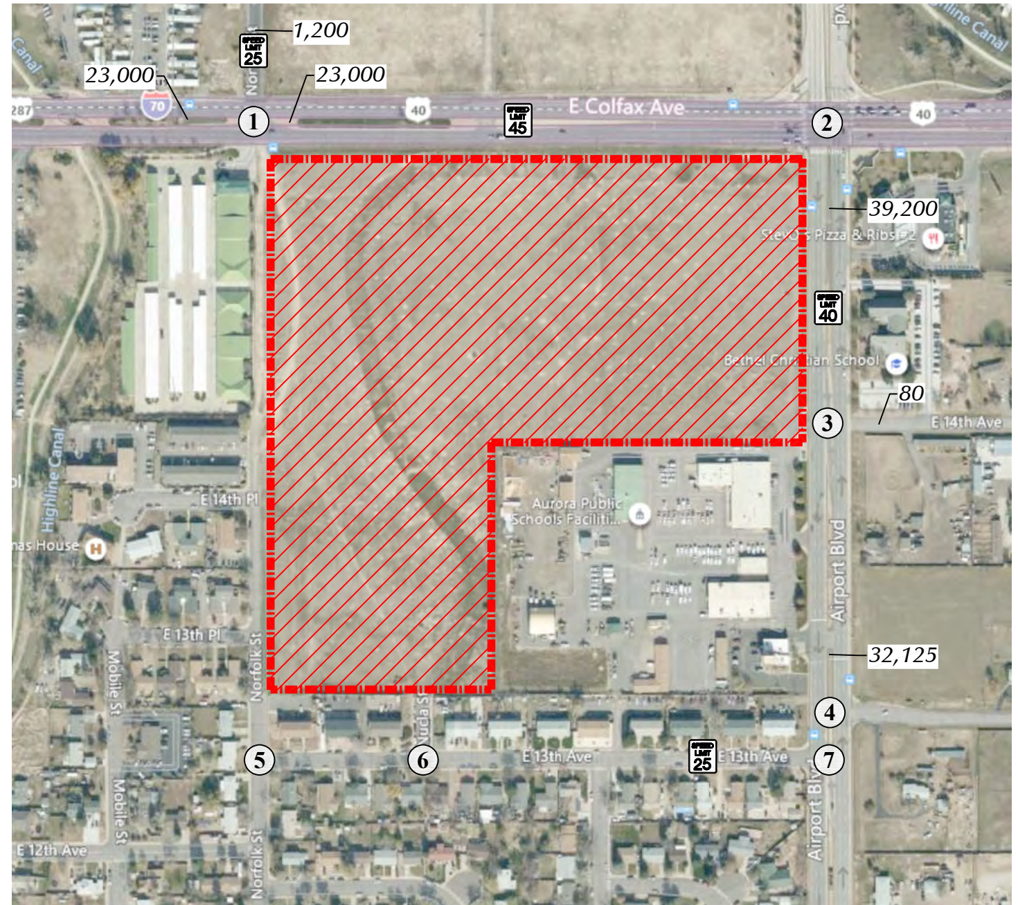
Figure 3 Existing Traffic, Lane Geometry and Traffic Control Salud Appeal of Station 60 ISP Decision (LSC #220010)
