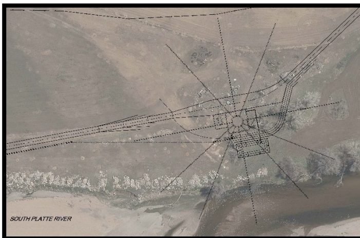
Top View of Caisson and Radials (subgrade)
