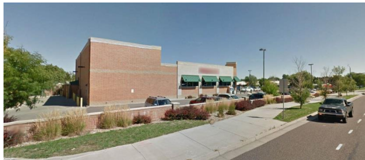
Figure 4.7-29: A Low Wall in Combination with Landscaping to Screen the Parking Lot
