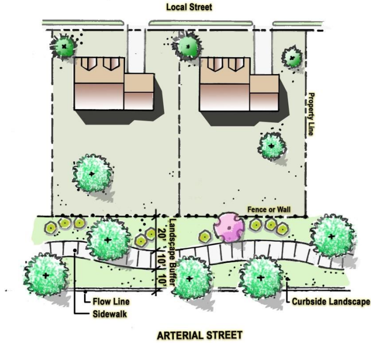
Figure 4.7-33 Arterial Street Frontage – Meandering Walk
